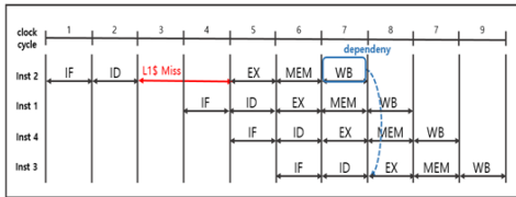
(그림 2) Out-of-Order execution.
